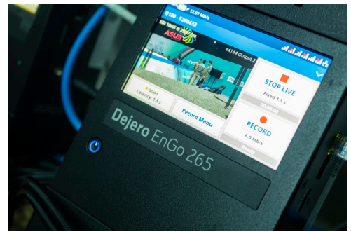
Each of Quality's 90+ cameras used a Dejero EnGo to transport live feeds from sports venues across Asunción to WayPoint receivers at the IBC and Quality's Buenos Aires hub.
