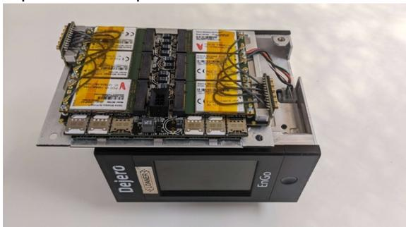
9. Orient the new SIM cards as shown in the picture below. The SIMs vary in design and may not have logos. It is important that this order is followed to ensure your device functions correctly.
