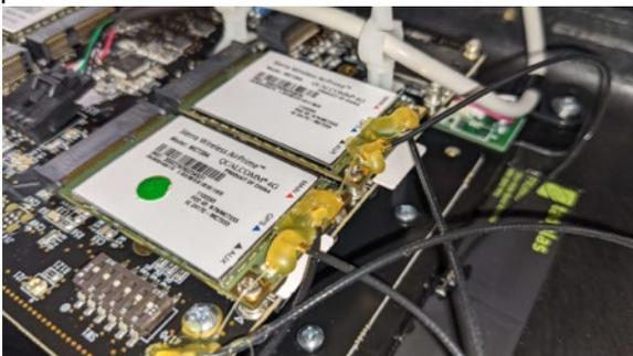
5. Replace each SIM by removing it gently, ensuring that the wires are not disturbed and become detached. If they become detached, they can be put back on and affixed with a small amount of hot glue.
