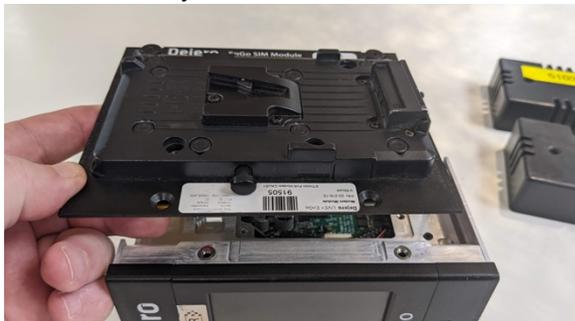
8. Flip the modem panel over and rest it on the chassis. This exposes the SIMs along the bottom edge.
