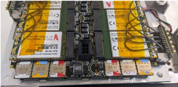
11. Reverse the disassembly instructions carefully placing the modem panel as shown so there are no exposed wires. Tuck them in before replacing the four screws.
