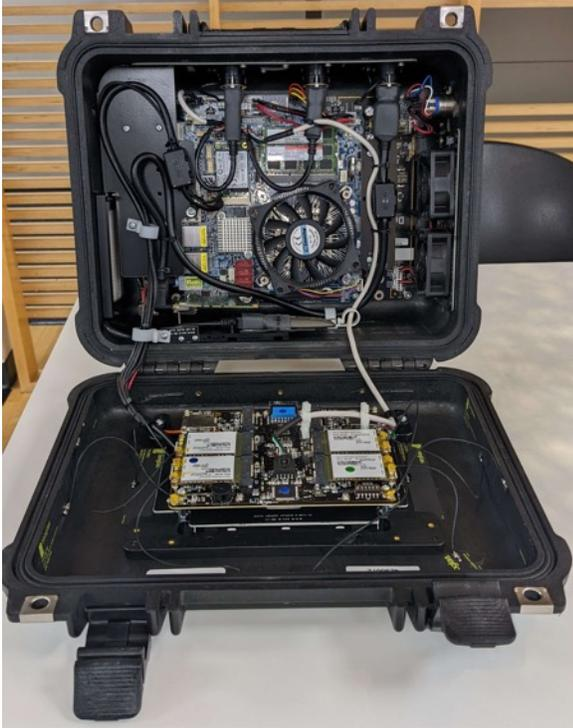
3. Locate the modems on the lid. The SIM cards will be visible under the modems.
