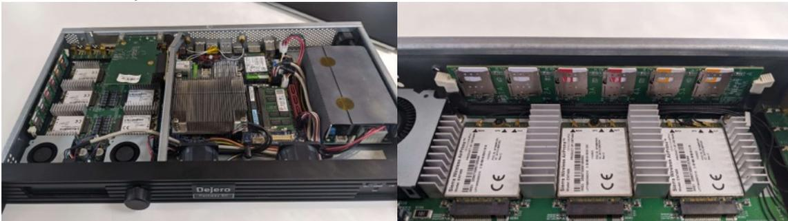
4. Swap the existing SIMs with the new ones we sent you. Ensure that each SIM is inserted into the proper SIM slot:
