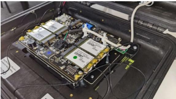
4. Press gently inwards on each SIM card to remove it. They are spring-loaded and will pop out halfway when pressed.
