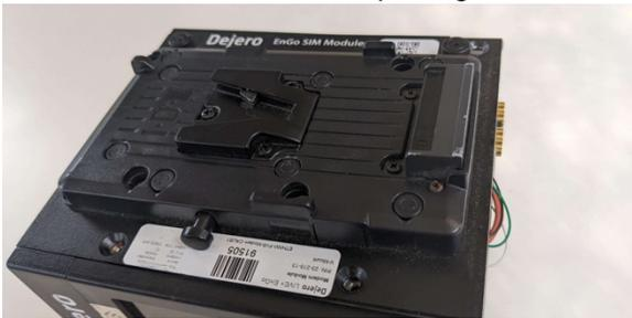
12. Place the caps back on the EnGo 1.x ensuring that the gold contacts are orientated correctly.
