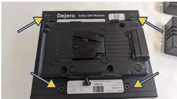
6. Using the #2 Phillips screwdriver, remove the four screws shown in the above picture.
